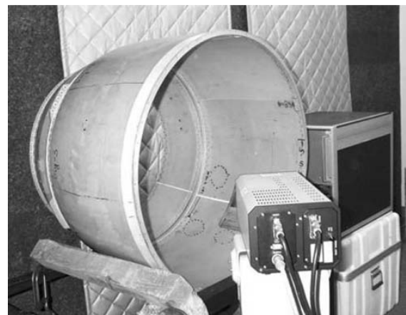
2 Jet engine casing undergoing testing: scanning LDV is in foreground and shockwave generator behind casing
