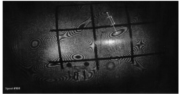
3 Specimen hologram used for calculation of velocity, strain and displacement
