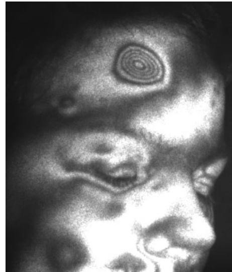
2 Circular fringe pattern clearly illustrates region of calvarial loss caused by bullet wound
